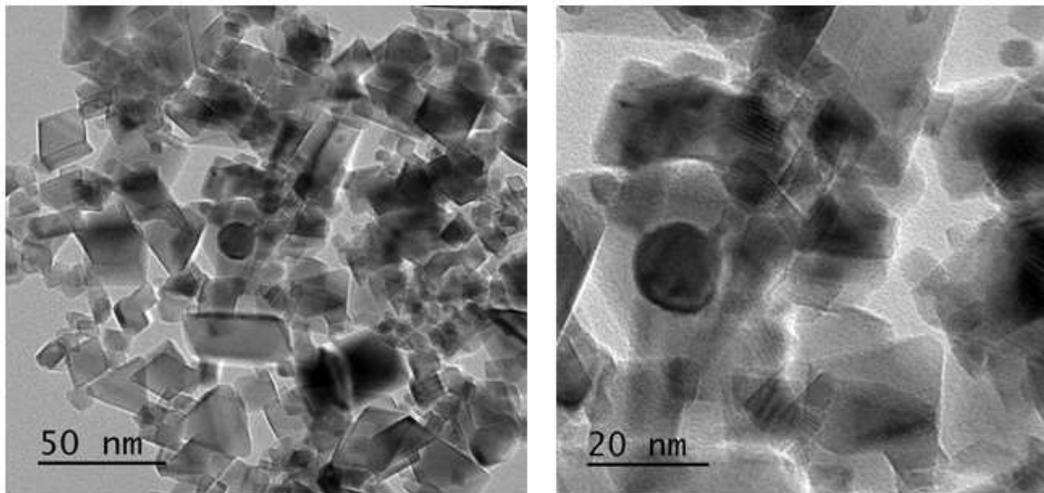
**Fig (2)** Cerium oxide nanoparticles TEM photomicrograph.
