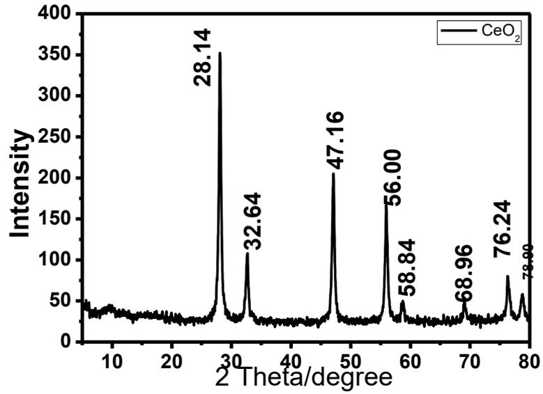
**Fig (1)** cerium oxide nanoparticles (XRD) analysis.
