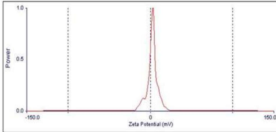
**Fig (3)** Cerium oxide nanoparticles zeta potential analysis, showing a peak at 1.5 mV.
