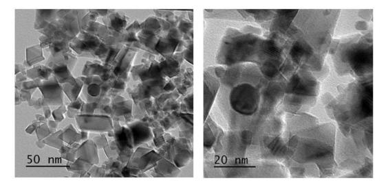
Fig (2) Cerium oxide nanoparticles TEM photomicrograph.
