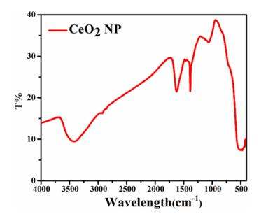
Fig (5) Cerium oxide nanoparticles (FTI) analysis.
