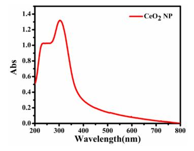
Fig (4) Cerium oxide nanoparticles (U-V) analysis.
