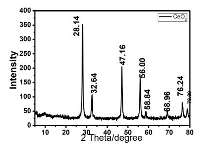
Fig (1) cerium oxide nanoparticles (XRD) analysis.
