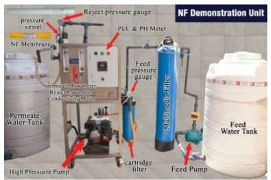
Figure 1. NF demonstration unit.
