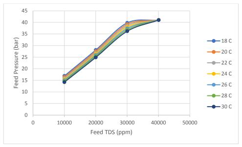
Figure 7. Effect of feed TDS on feed pressure.
