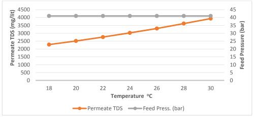
Figure 2. The effect of the feed temperature on both permeate salinity and the feed pressure at feed TDS 40K ppm by NF90-2540 at 40000 mg/L.
