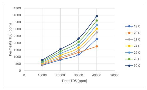
Figure 6. Effect of feed TDS on permeate TDS.
