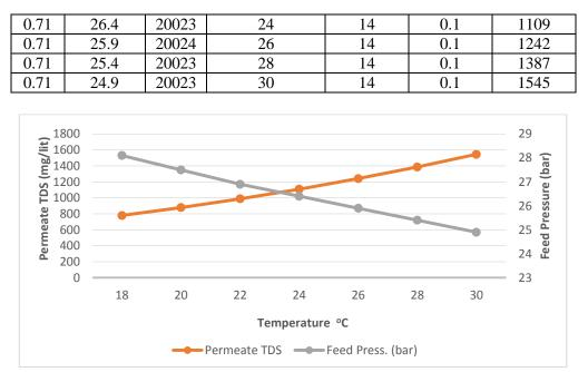
Figure 4. The effect of the feed temperature on both permeate salinity and the feed pressure at feed TDS 20K ppm by NF90-2540 at 20000 mg/L.
