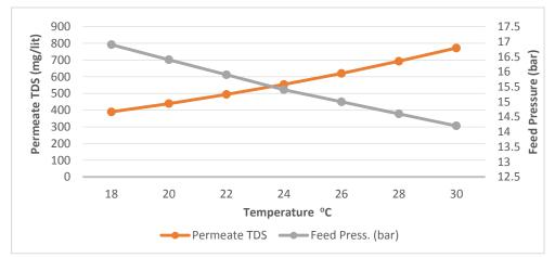
**Figure 5.** The effect of the feed temperature on both permeate salinity and the feed pressure at feed TDS 10K ppm by NF90-2540 at 10000 mg/L.
