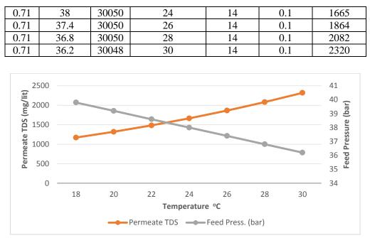
**Figure 3.** The effect of the feed temperature on both permeate salinity and the feed pressure at feed TDS 30K ppm by NF90-2540 at 30000 mg/L.
